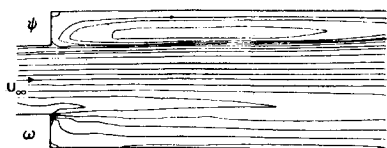
Fig. 12a Computed steady-state streamfunction and vorticity for flow over a rearward step, Re = 200 .
